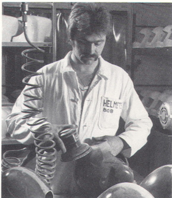
Bob Waller buffing motorcycle shells in the GRP moulding shop. At the back, crash tender and industrial helmets.
