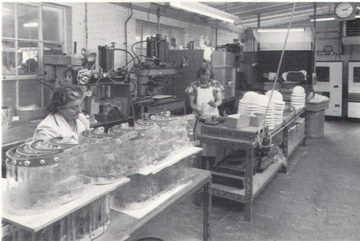
Barbara Smith fitting out polycarbonate riot visors, which are formed in the ovens in the background; and beyond her, Ronnie O'Grady working at a bench loaded with agricultural spray guards for RFD. The visors are covered with a protective film.
