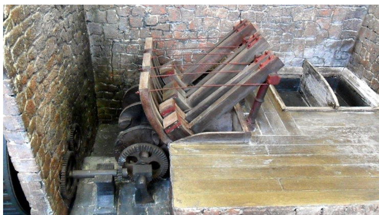
The hammers and cog wheels of a fulling mill
